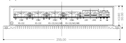
Figure 2.1: Front panel of UNO-2170
